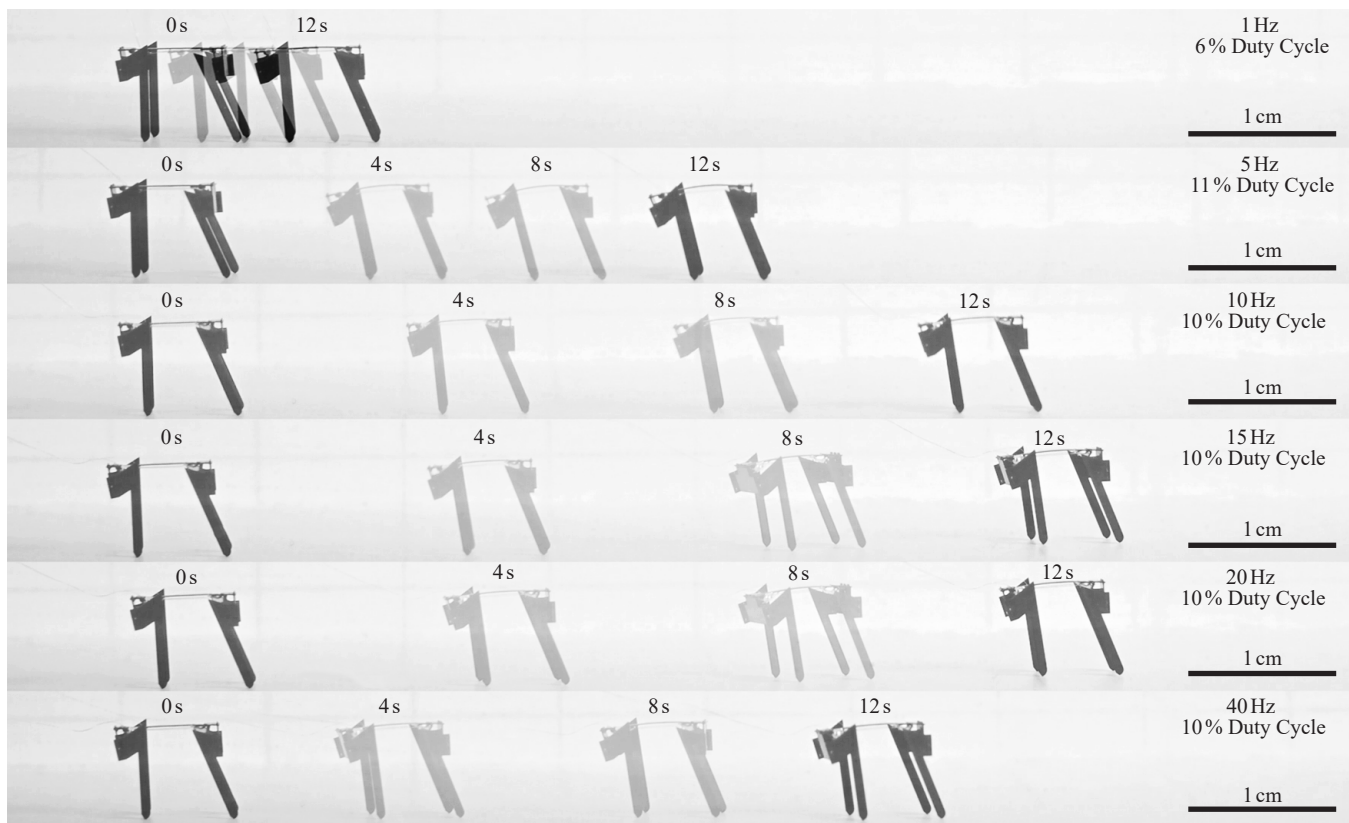
Fig. 8. The MiniBug locomoting at six different actuation frequencies. The photographic sequences show the distance traveled by the MiniBug at intervals of 4 s, for the operation frequencies in the set \{1, 5, 10, 15, 20, 40\} Hz; the DC values are the empirical optima determined according to the method discussed in Section III. The fastest relative speed of 0.76 BL/s occurs at 15 Hz. Depending on the frequency of operation, the robot exhibits four locomotion modes: (i) crawling , (ii) shuffling , (iii) galloping , and (iv) gliding . At 1 Hz, the MiniBug slowly crawls, achieving an average speed of 0.10 BL/s; at 5 Hz, the locomotion mode changes to shuffling, during which the MiniBug achieves an average speed of 0.46 BL/s; at 10 Hz, 15 Hz, and 20 Hz, the locomotion mode switches to galloping, during which the MiniBug achieves average speeds of 0.69 BL/s, 0.76 BL/s, and 0.75 BL/s, respectively. At the highest frequency of 40 Hz, the MiniBug glides and hardly any actuator output displacement can be noticed as high-frequency vibrations allow the robot to virtually float forward at an average speed of 0.61 BL/s. Video footage of these tests can be seen in the accompanying supplementary movie.
